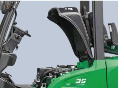
The hood can be opened at a large angle facilitating the maintenance.
